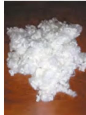
Figure 2 – Fiber of 6DE64 brand (manufactured in Korea)
