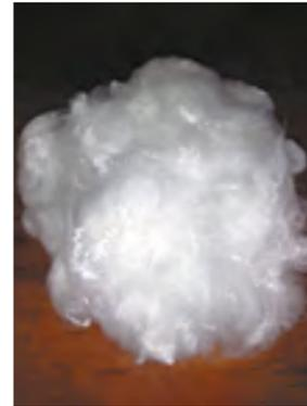
Figure 1 – Fiber of 4DE51Slon brand (manufactured in Korea)
