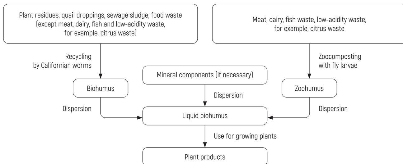
Figure 15 – Diagram of processing solid food waste to obtain plant products
