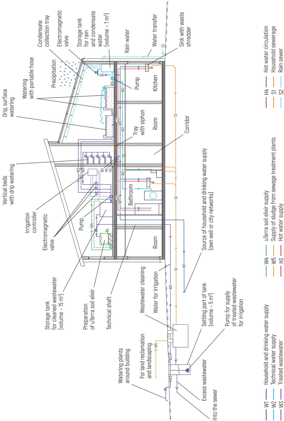
Figure 14 – Diagram of water reuse in a multifunctional building (variant)
