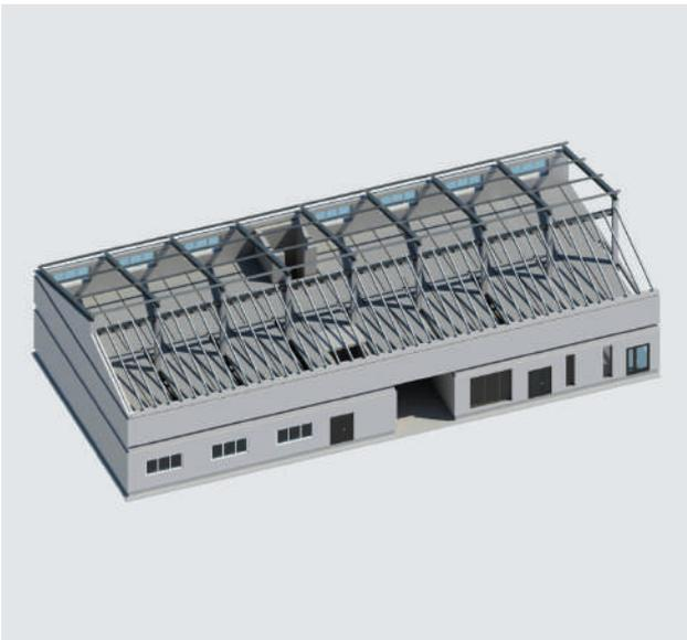
Figure 11 – Structural diagram of a multifunctional building made of prefabricated elements (fragment, variant)
