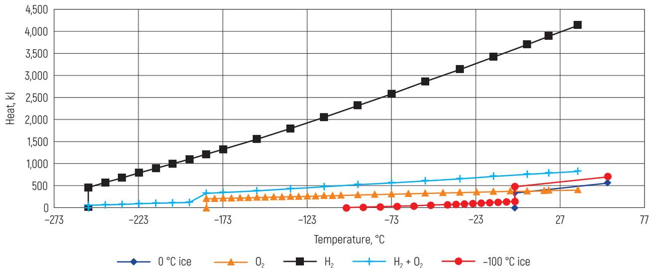
Figure 3 - Dependence of heat absorbed by the refrigerant on temperature
