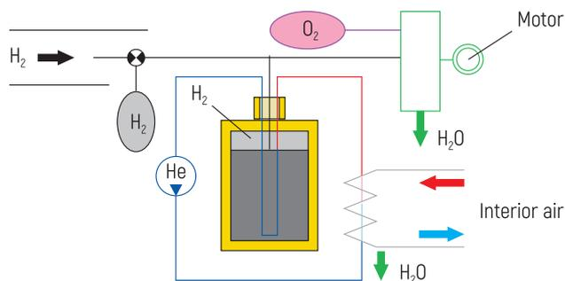
Figure 7 – Working diagram of the hydrogen heat converter
