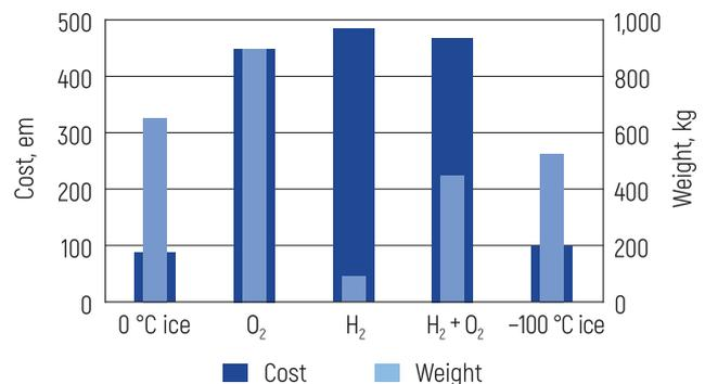
Figure 5 – Cost and weight of the refrigerants in the battery per one HV trip
