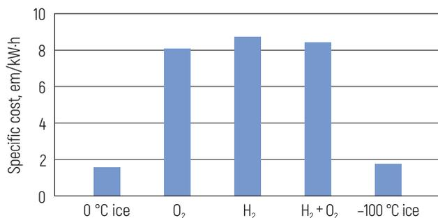
Figure 6 – Specific cost of the refrigerants per 1 kW-h of electrical energy consumption per one HV trip
