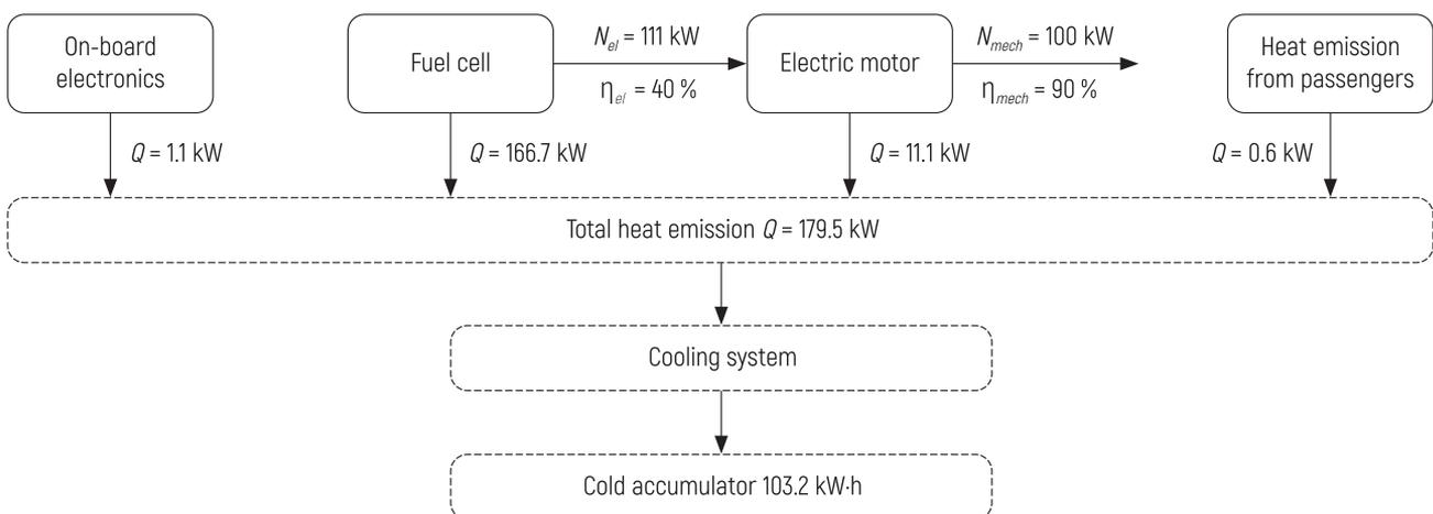
Figure 4 - Flows of excess thermal energy of the HV and their estimated capacity
