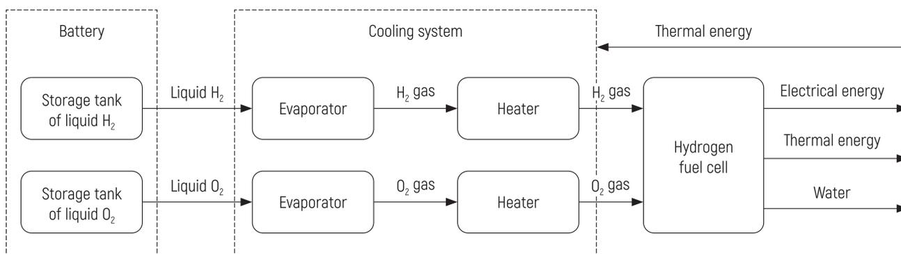
Figure 2 – Diagram of the use of hydrogen and oxygen as a refrigerant and energy sources on board the HV
